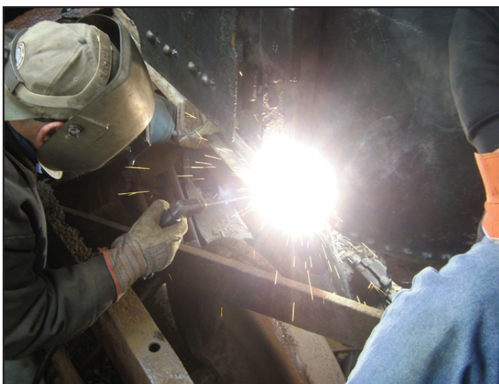
Bob Pitcher is welding angle iron in the above photo by Joseph Alves, and the new custom-built tender floor shown in the photo below shot by Carolyn Taylor.
