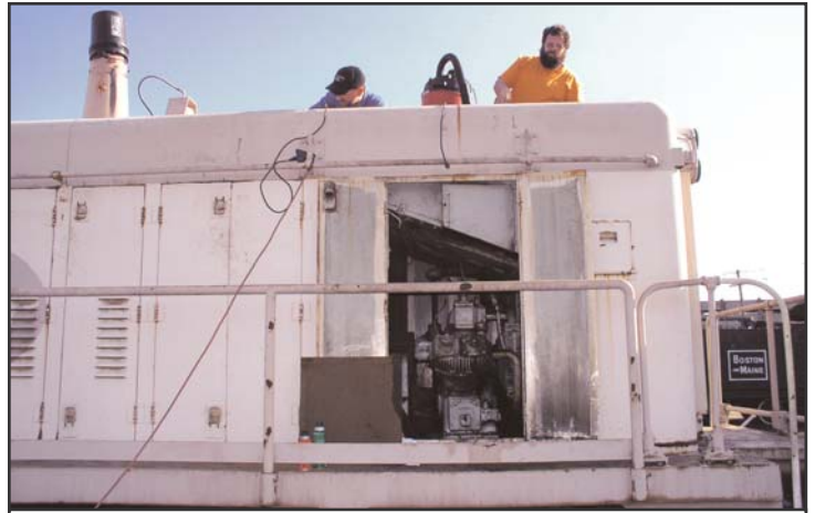
Dan Carleton and Justin Chapin have been working hard and late to remove corrosion from inside the SW8. With the radiator bank temporarily removed, they have access to that area, and will protect it with paint it before installing the new radiator bank.
